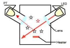
Figure 1 - Model of dust sensor
