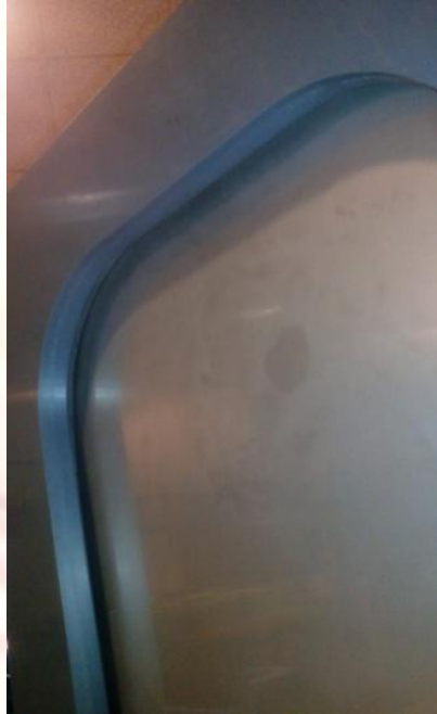
Membrane in groove of the PVC bottom for closing /opening
